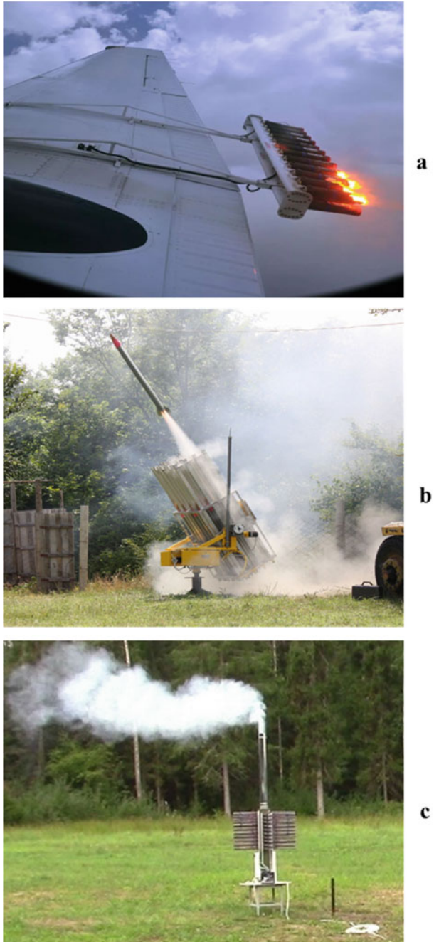
Fig. 2.3 Technical systems for delivering seeding materials into clouds and their environments: a airborne pyroflares; b small-sized anti-hail rocket “Alazan-6” and automated anti-hail launcher “ELIA-2”; c liquid acetone-based ground generator. Sources a National Center of Meteorology of the United Arab Emirates; b Magomet Abshaev; c Viktor Korneev; all used with permission
