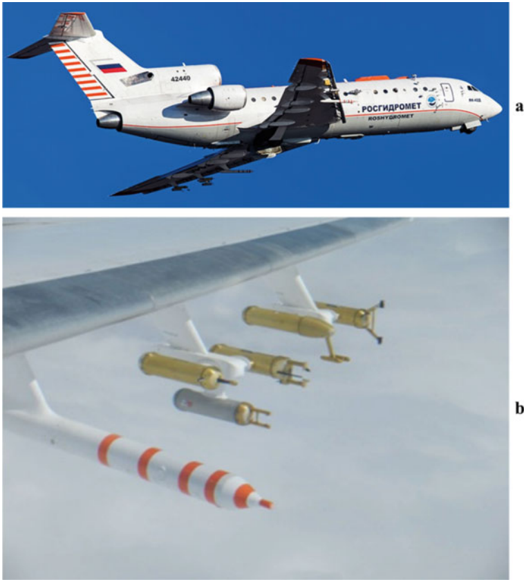
Fig. 2.4 Highly equipped middle-sized research aircraft “ROSHYDROMET YAK-42D” of the Russian Hydrometeorological Service for measurement of atmospheric and cloud characteristics and cloud seeding, using various types of seeding materials: a external view; b sensors for aerosol, cloud droplets, and ice crystals spectrum, temperature, humidity, water content. Source Viktor Petrov; used with permission
